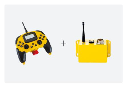
The Safe Remote Control pairs with FORT's Vehicle Safety Controller receiver (VSC).
